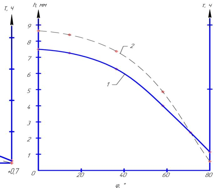
Fig. 7 - Dependence of the height (1) and time (2) of the capillary rise of the binder on the wetting angle of the base by the binder
