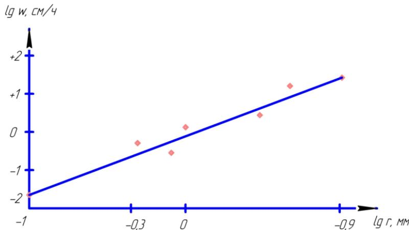
Fig. 10 - Dependence of the settling velocity of particles with a radius of 0.1 ÷ 8 mm in petroleum pitch
