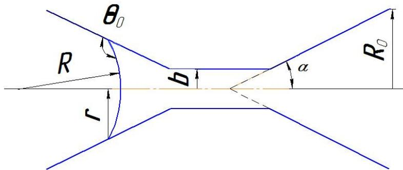
Figure 8 – Schematic of a narrowing - expanding pore
