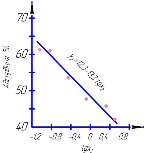
Fig. 12 - Dependence of adsorption capacity of powders on particle size
