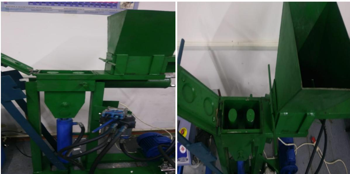
**Fig. 5 - Pilot plant for briquette production**
