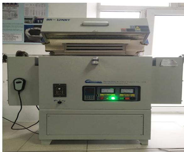
Fig. 1-High-Temperature Rotary Tube Furnace BR-12NRT
