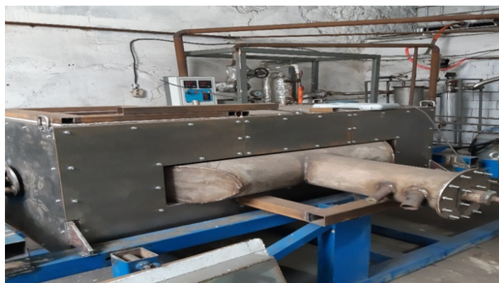
Figure 1 - Pilot-scale rotating drum furnace for thermal treatment of semi-coke fines
