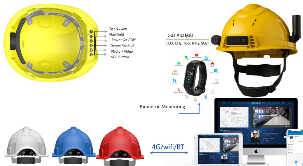
Fig.1 - Functional diagram and capabilities of the intelligent helmet
